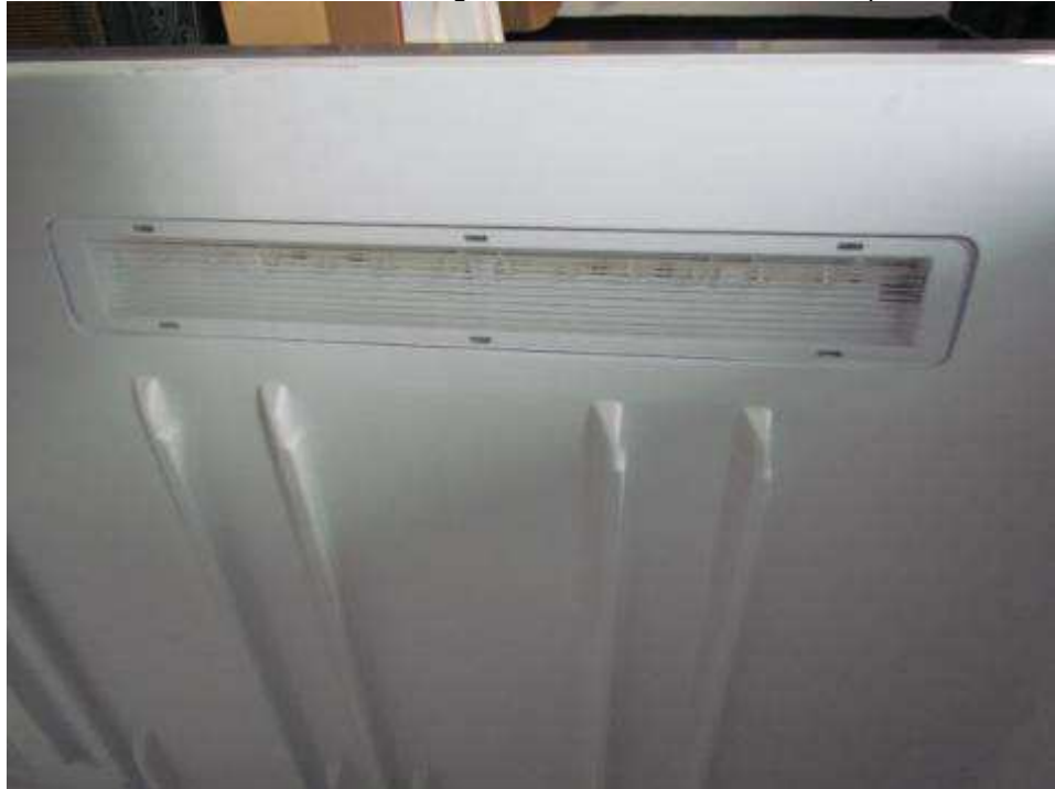
LED lamp placed beside of compartment
