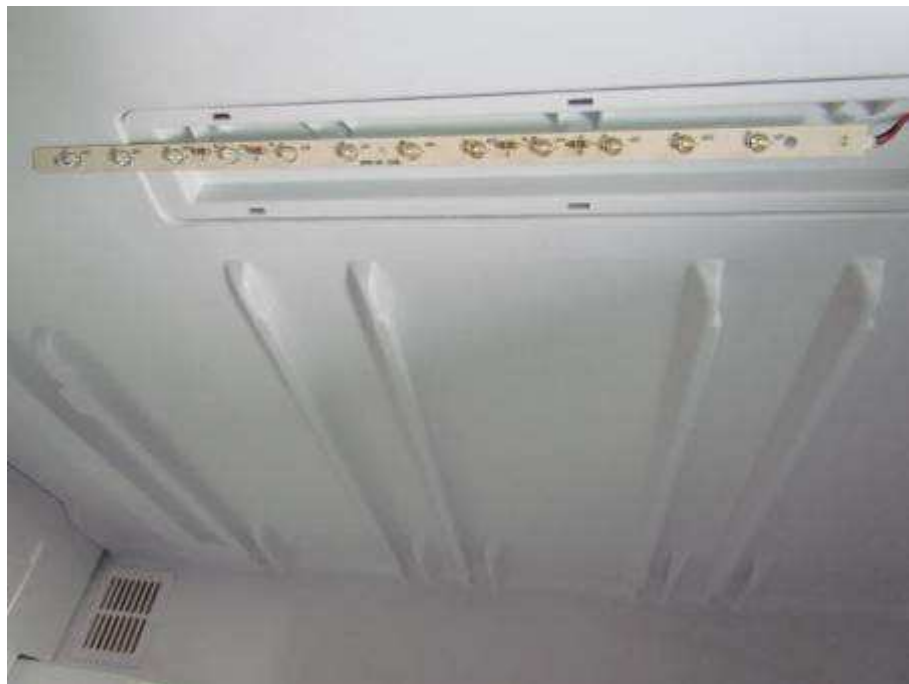
LED lamp placed beside of compartment
